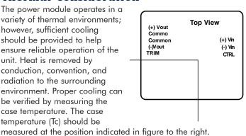
When operating the module, adequate cooling must be provided to maintain the case temperature at or below 100°C. Maintaining a lower temperature will yield higher reliability of the device. Optimum cooling is obtained with forced convection.
